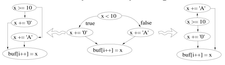
we may reorder basic blocks of a control flow graph of every function to make the most frequent jumps be "fall-through"
