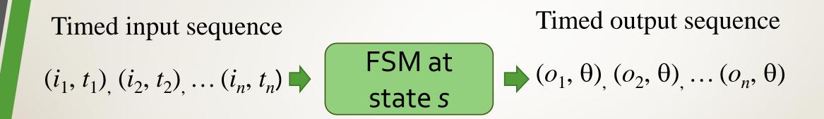
S is a deterministic complete (Timed) FSM if for each pair (*s*, *i*)  $\in S \times I$ , there is exactly one transition (*s*, *i*, *o*, *s'*)  $\in h_S$
