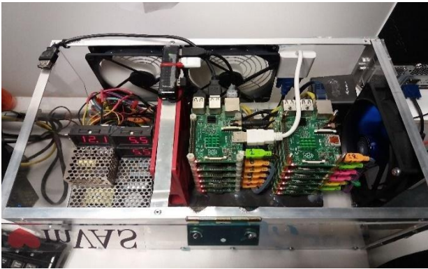
Fig. 1. Construction of Beowulf Cluster [11]
