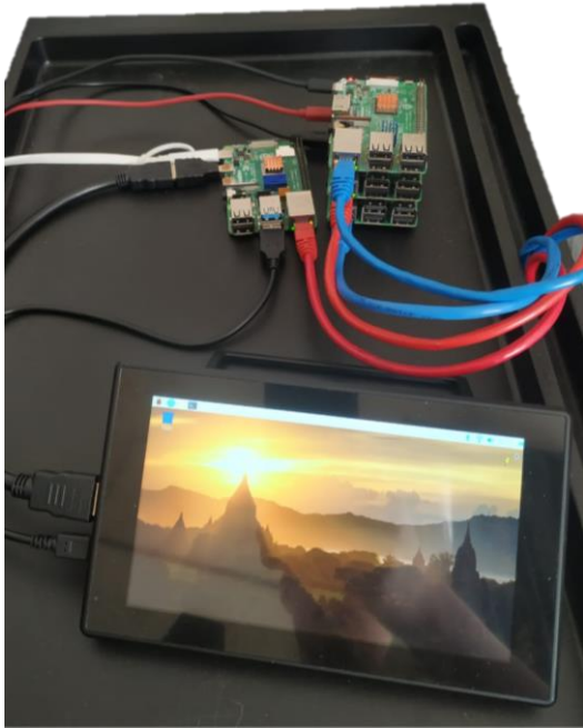
Fig. 4. Example of an assembled system of four nodes.
