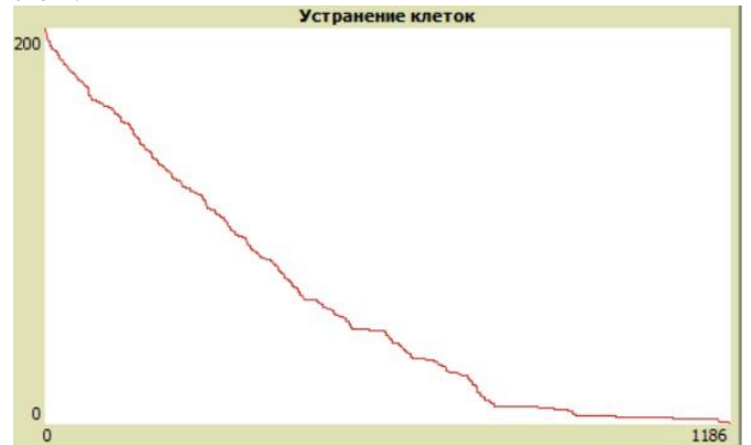
Fig. 6. Graph of the dynamics of the change in the number of cells ( the number of robots is 200; the number of cells is 200, the radius of the aura-signal is 41 patches.)
