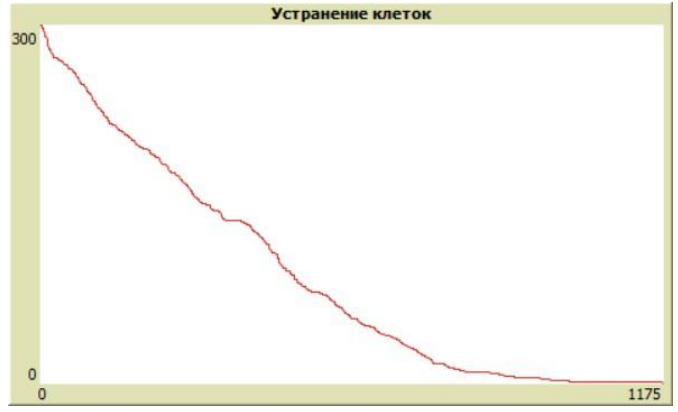
Fig. 5. Graph of the dynamics of changes in the number of cells ( the number of robots is 200; the number of cells is 300, the radius of the aura-signal is 10 patches)
